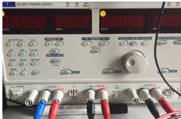
Figure 3.3: First power supply, used for the active parts of the circuits.
