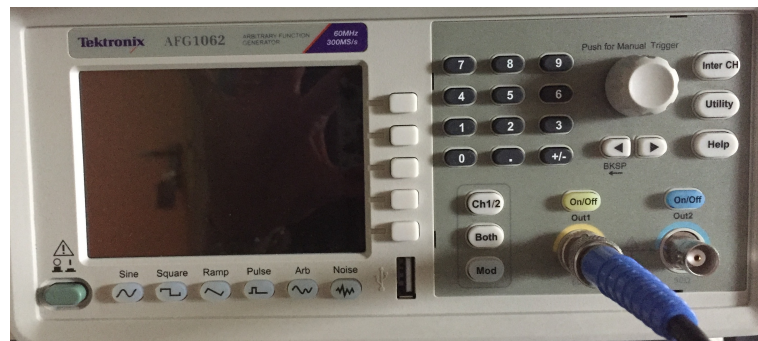
Figure 3.5: Function generator, is used for simulating the signal coming from the diode or other parts of the circuit.
