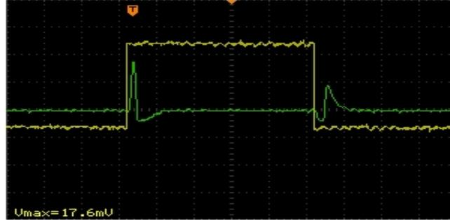
FIGURE 4.6: Combination between the pulser peaks (the yellow peak) and the same peak after main amplifier (green one).
