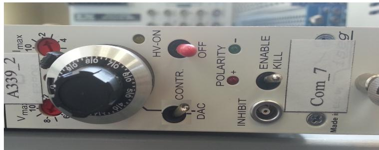
FIGURE B.9: The control button of the power supply
