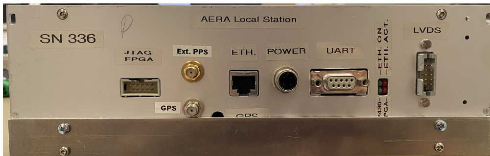
Figure 4.16: The front panel of an AERA digitizer that has been modified. A SMA connector for the external PPS input has been added to connect a WR to the digitizer and the position of the SMA input for the GPS antenna has been moved because the extension of the front panel covers a part of the previous hole for the GPS.
