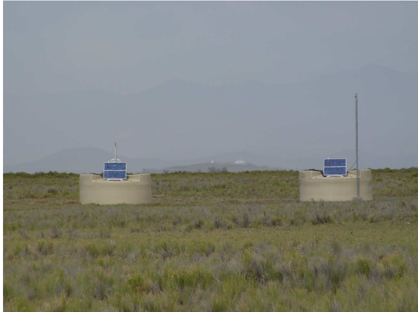
Figure 9: The Surface Detector stations “Carmen” and “Miranda”, the first SD stations working in pair tank configuration. The FD site of Los Leones can be seen in the background [22].
