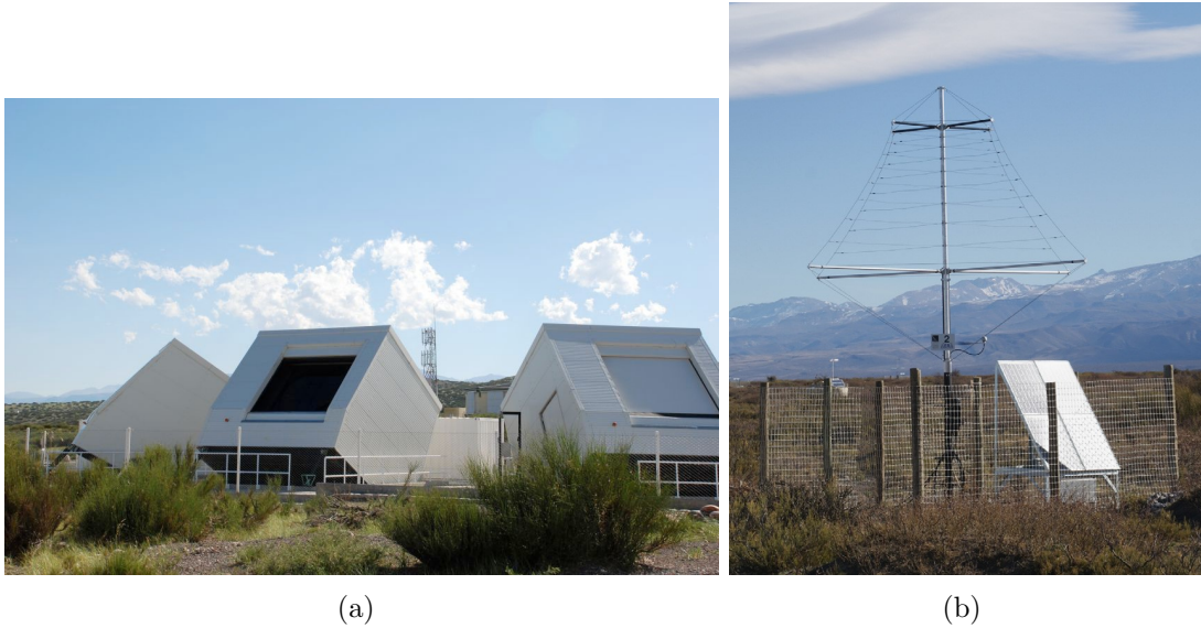
Figure 3.5: (a) The three HEAT telescopes tilted upward [33]; (b) a radio detector station installed at the AERA site [34].
