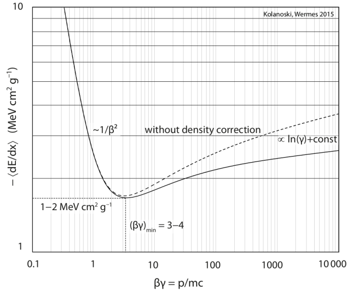
Figure 2.5: The mean energy loss of a charged particle by ionisation as described by the Bethe-Bloch equation [3, p. 39].
