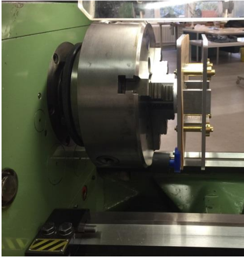
Figure 4.2 The coil frame mounted on winding spindle of a winding machine. The winding frame along with wire guide (not shown in the figure) ensures orthocyclic winding.
