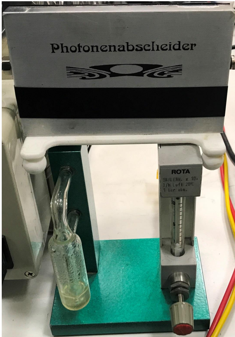
Figure 4.27 Air from the pump enters the dehumidifier and then travels through photon absorber before reaching the detector enclosure.
