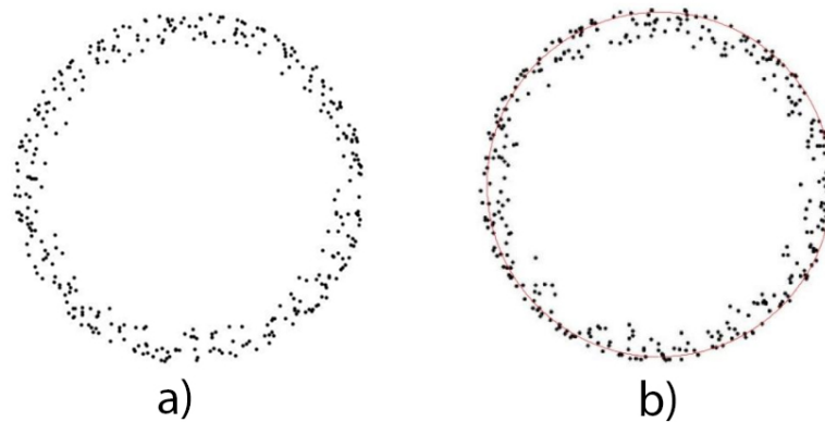
Figure 3.9: Panel a shows the raw data set passed to the CHT whereas panel b shows the detected circle drawn in red.
