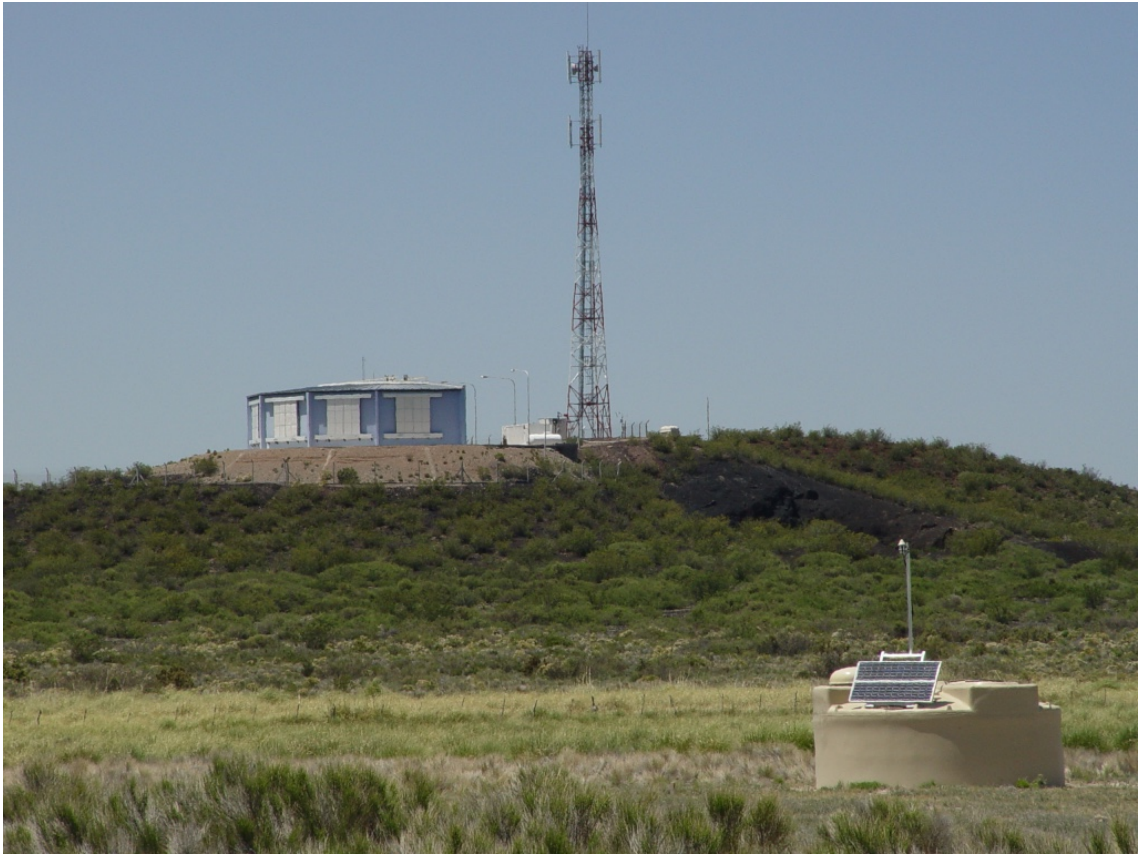
Figure 4.2.: Photograph of a water Cherenkov detector station from the SD of the Pierre Auger Observatory in front of one of the four FD sites [24].
