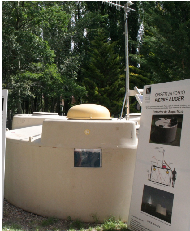
Figure 2.2.: This SD-Tank is placed in front of the main building of the Pierre Auger Observatory. It is not filled with water and has a window in the front to let visitors see the inside of a tank (Picture: private).
