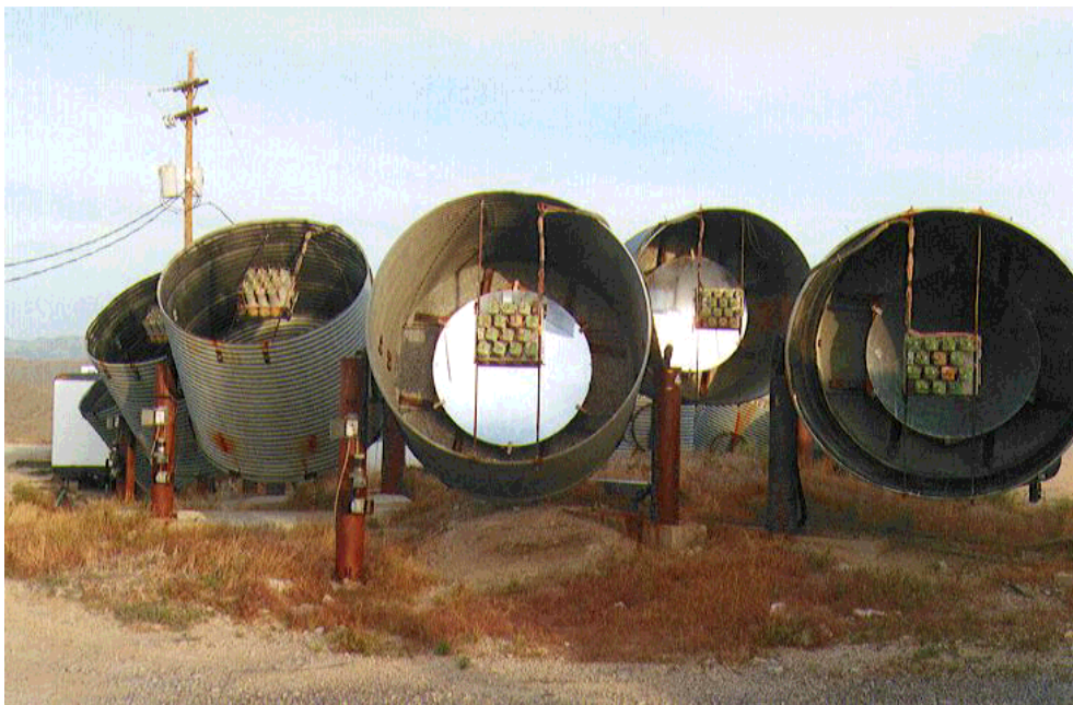
Figure 7.30: Arrangement of mirrors and photomultipliers in the original Fly's Eye experiment of the Utah group {25}
